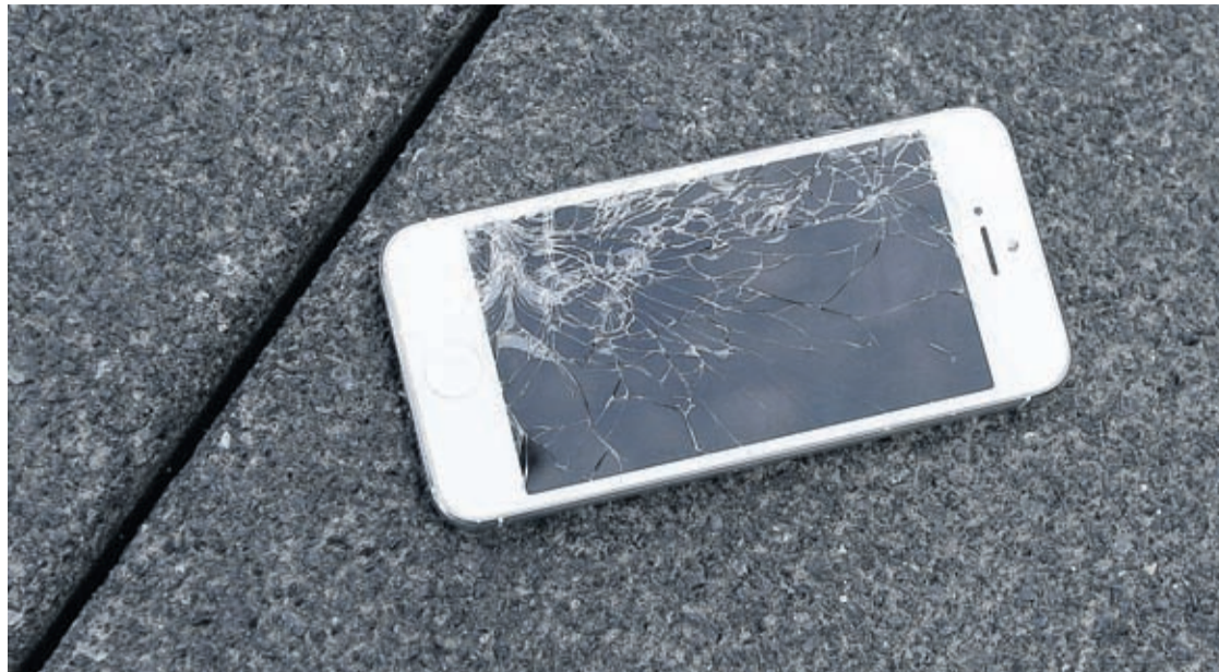
This Aug. 26, 2015 photo shows an Apple iPhone with a cracked screen after a drop test from the DropBot, a robot used to measure the sustainability of a phone to dropping, at the offices of SquareTrade in San Francisco.
